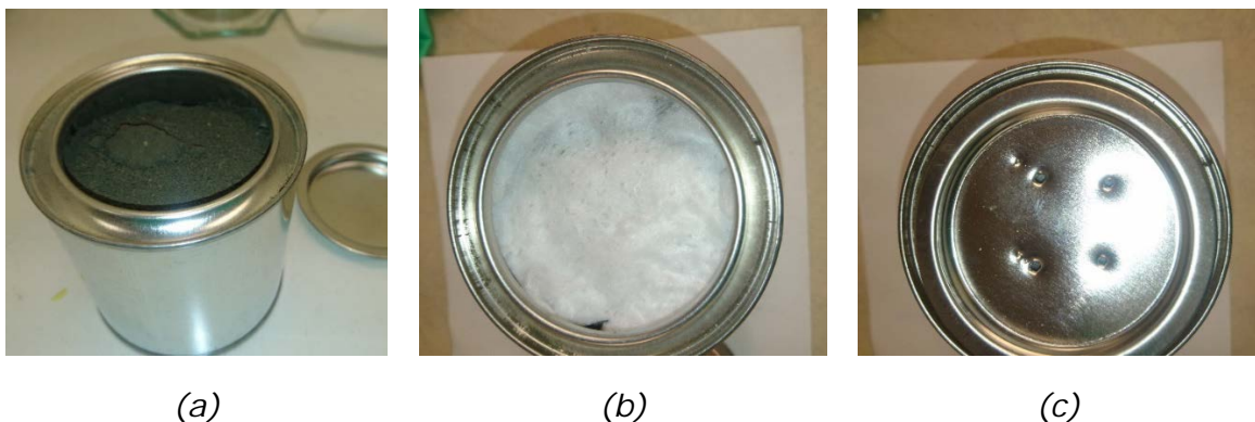
Fig. 3. (a) Container filled with dry solid, (b) filter and (c) holes in the lid for evacuation of air.
