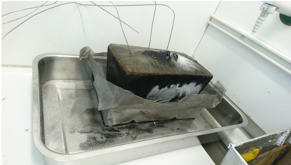
Fig. 6. Thawing of frozen sludge
