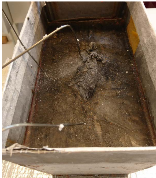
Fig. 5. Frozen sludge prior to thawing, with visible thermocouples
